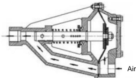
Automatic Air-Venting Valve is Open
