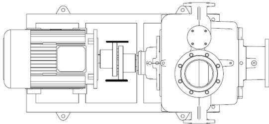
**(Figure 3-3) Parallel Sliding Error in Horizontal Plane**
