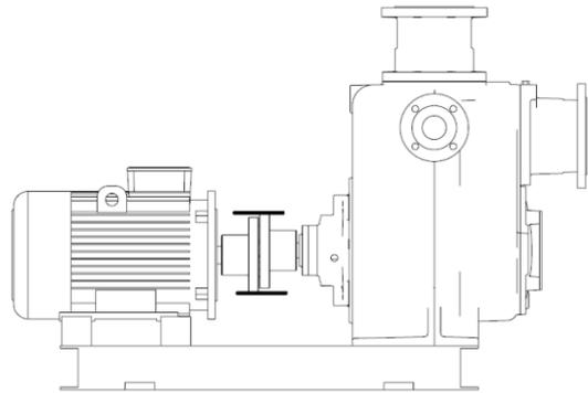
**(Figure 3-4) Parallel Sliding Error in Vertical Plane**
